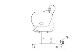
2. Fully insert and attach the short basket hooks to the upper guides of base upright left and right.
