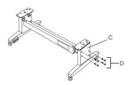
4. Fasten eight screws on the both sides of the base upright securely.
