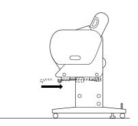
3. Likewise, fully insert and attach the long basket hooks to the lower guides.
