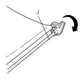
9. Slide out the lower basket hooks to their full length, then attach the L shape ends to the joint sockets (K) on the front side.
