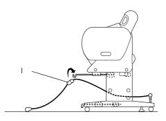
8. Hold the front side shafts (J) and turn it one revolution as shown below.
