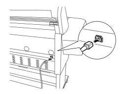
2. Attach the three clamps packed with your printer, then route the power cord through the clamps at the rear of the printer.
