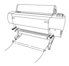
7. Hook the both ends of the center shafts (I) on the upper basket hooks.
