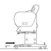
4. Turning the stitch side downward, spread the paper basket on the floor.
