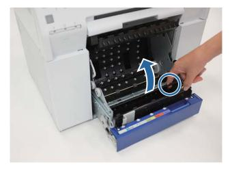
10 Check that there is no paper, foreign material, or scrap paper at the back of the printer.
