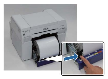
5 Insert the leading edge of the paper into the paper feed slot.
