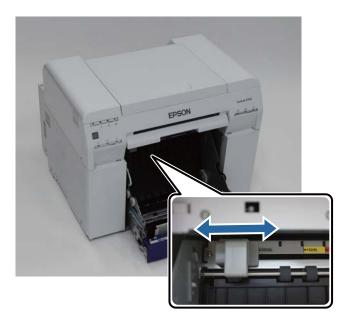
2 Hold the spindle unit in the direction shown below, and then place it in front of the roll paper feeder. Remove any tape or protective sheets from the paper. If the leading edge of the paper is ragged, cut it in a straight line with a pair of scissors and so on.
