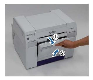
Grip the handle to release the lock, and then pull out the roll paper feeder.
