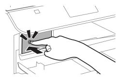
3. Remove the ink cartridge from the printer.
