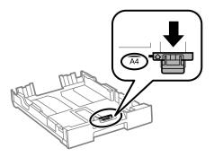
4. With the printable side facing down, load paper against the front edge guide.
