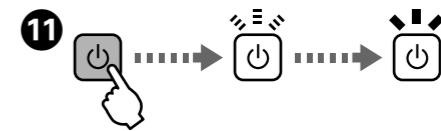
Turn on the printer and wait until the light stops flashing.
