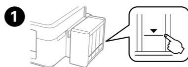
Visually check the ink levels of all ink tanks. If the ink level is below the lower line on the tanks, go to step **2** to refill the tanks.
