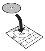
7. Insert the CD/DVD tray into the printer. Line up the alignment marks on the printer and the tray.
