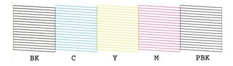
☐ There are broken lines or missing segments: The print head nozzles may be clogged. Go to the next step.
