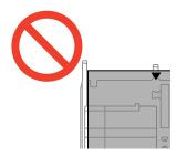
□ Do not load more than the maximum number of sheets specified for the paper. For plain paper, do not load above the line indicated by the triangle symbol on the edge guide.
