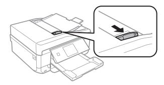
4. Place the originals face-up in the ADF, and then slide the ADF edge guide to the edge of the originals.
