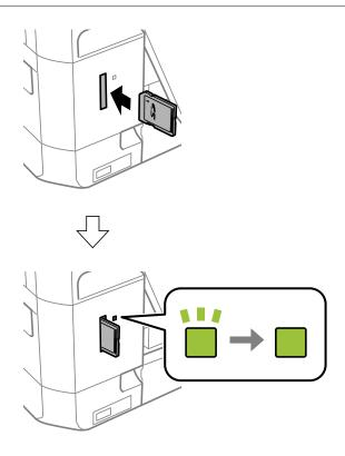
When you have finished using the memory card, make sure the light is not flashing, and then remove the card.
