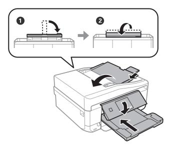
10. Pack the printer in its box, using the protective materials.
