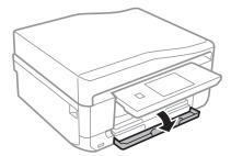
Check that the printer is not operating, and then pull out paper cassette 1. Paper cassette 1 has an alignment mark that allows you to locate it easily.
