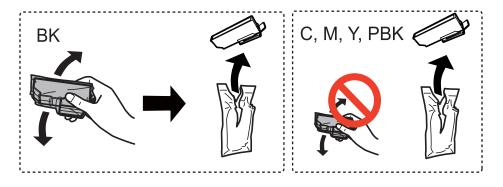
☐ Do not shake cartridges after opening the package, as they may leak.
