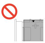
□ Do not load more than the maximum number of sheets specified for the paper. Do not load paper above the line indicated by the triangle symbol on the edge guide.
