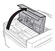
2. Use a soft, dry, clean cloth to clean the roller and the interior of the ADF, and then close the ADF cover.
