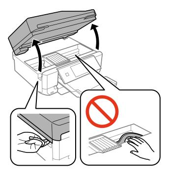
5. Push the tab to unlock the ink cartridge holder, and then remove the cartridge diagonally.
