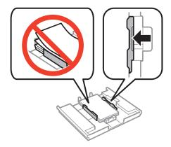
8. Insert paper cassette 1. Line up the alignment marks on the printer and the tray.
