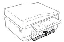
5. Remove the CD/DVD tray from the bottom of the printer
