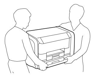
☐ When carrying the printer, do not tilt it more than 10 degrees; otherwise the printer may fall.
