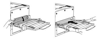
When the paper jam is cleared completely and the paper path unit (unit C) is pushed back into the printer, the jammed page's print data is automatically reprinted.
