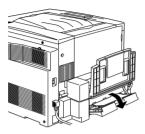
Gently remove the jammed paper inside the inverter cover.
