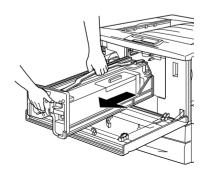
Take the new photoconductor unit out of its package and unwrap the protective sheet while holding the handle as shown below.
