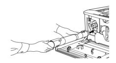
Turn the toner cartridge knob 90 degrees clockwise so that the O symbol on the knob is in the position shown below. By turning the knob, the cartridge is pressed into the slot and installed completely.
