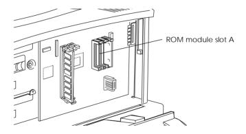
12. Insert the module all the way into slot A as shown below.
