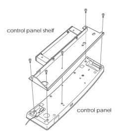
3. Insert the control panel shelf straight into the opening on the front of the cabinet's top panel.
