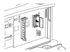
13. Make sure the tab on the left of the slot shown below will stick out when the module is inserted correctly.
