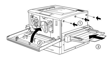
16. Install the large capacity paper unit or 500-sheet paper cassette unit as explained in the printer's manual.
