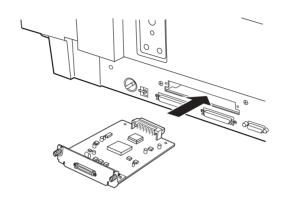
5. Secure the board with the retaining screws.
