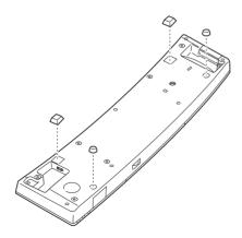
Plug the shielded control panel cable into the control panel's interface connector, located on the bottom of the control panel.
