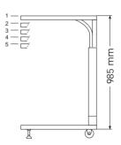
The stand height is adjustable to five positions. When the stand is in position 3, 4, or 5, use holes A to fasten joint B.
