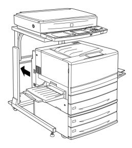
18. Lock all casters on the bottom of the large capacity paper unit or 500-sheet paper cassette unit.
