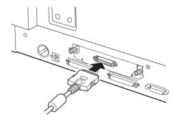
4. Plug the other end of the cable into the connector on the printer.
