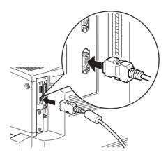
3. Plug the scanner cable into the scanner's interface connector.
