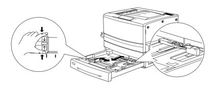
4. Fan a stack of plain paper and insert it into the cassette. Make sure that all the paper is under the retaining clip on the right side of the cassette.
