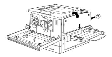
15. Secure the right cover with the screws, then close the front cover and push the paper path unit back into the printer.
