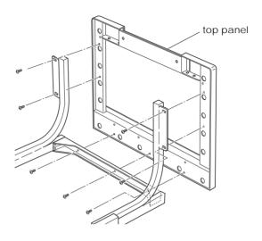
6. Fasten joint B to the frame with eight M4  $\times$  10 screws. Then securely fasten joint A, which was installed in step 3.
