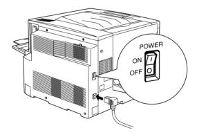
4. Plug the other end into a properly grounded electrical outlet.
