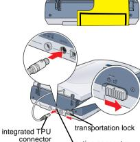
4. Connect the power cord and AC adapter, as shown. 5. Connect the AC adapter to the DC
