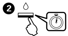
Run the print head cleaning. Hold down for **3 seconds** until starts flashing.
