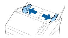
3. Load the plastic cards into the input tray facing down with the top edge facing into the ADF. Slide the plastic cards into the ADF until they meet resistance.
