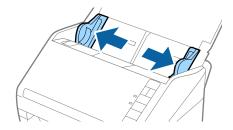
3. Load the envelopes into the input tray facing down making sure that the opened edge (flap side) of the envelope is facing to the side. For envelopes with the opened edge (flap side) on the shorter side, you can load the envelope with the opened edge (flap side) facing up.
