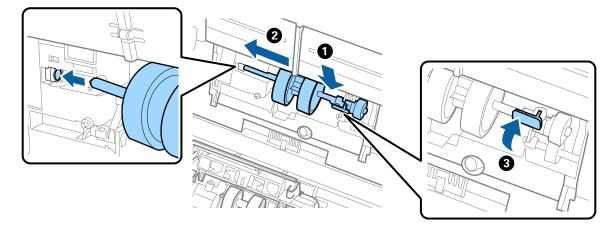
7. Put the edge of the cover of the pickup roller into the groove and slide it. Close the cover firmly.
