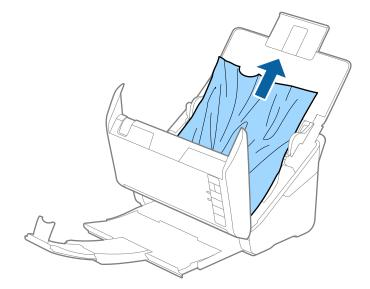
4. Carefully pull out any jammed originals from the output tray in the direction of the arrow if you cannot pull originals straight up.
