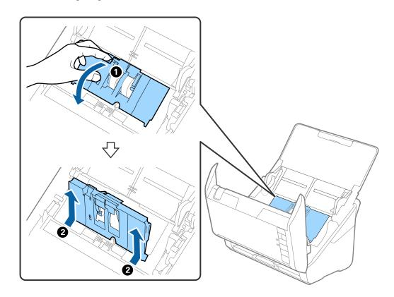
4. Open the cover of the pickup roller, and then slide and remove it.
