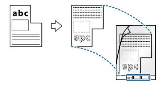
4. Load the Carrier Sheet into the input tray with the top edge facing into the ADF. Slide the Carrier Sheet into the ADF until it meets resistance.
