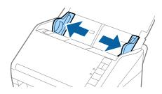
3. Place the Carrier Sheet with the illustration on the front edge facing up and place the original in the carrier sheet by folding it in half so that the side to be scanned is facing out, with the right side at the front.
