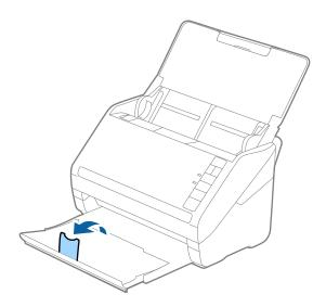
2. Slide the edge guides on the input tray all the way out.
