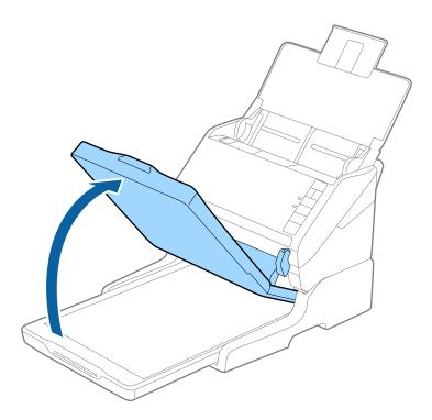
3. Place your document or photo face down on the scanner glass making sure the upper corner of the side you want to scan is against the corner of the scanner next to the arrow mark.
