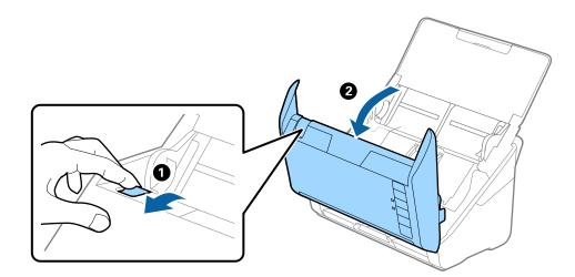
3. Carefully remove any originals remaining inside the scanner.
