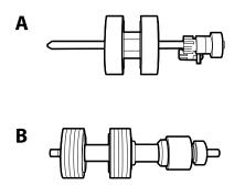
A: pickup roller, B: separation roller
