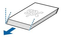
5. Load the originals into the input tray facing down with the top edge facing into the ADF. Slide the originals into the ADF until they meet resistance.
