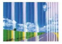
The print head nozzles may be clogged. Perform a nozzle check to check if the print head nozzles are clogged. Clean the print head if any of the print head nozzles are clogged.
