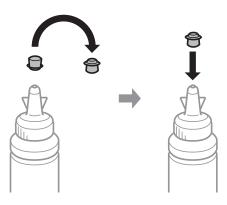
9. Close the cap onto the ink tank securely.
