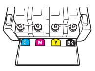
7. Snap off the top of the cap, remove the cap of the ink bottle, remove the seal from the bottle, and then install the cap.
