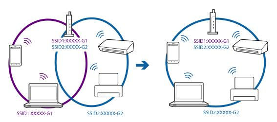
□ An access point that is compliant with both IEEE802.11a and IEEE802.11g has SSIDs of 2.4 GHz and 5 GHz. If you connect the computer or smart device to a 5 GHz SSID, you cannot be able to connect to the printer because the printer only supports communication over 2.4 GHz. Connect the computer or smart device to the same SSID as the printer.
