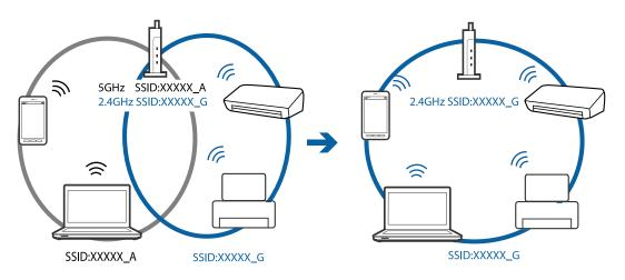
Most access points have a privacy separator feature that blocks the communication from unauthorized devices. If you cannot connect to the network even if the devices and access point are connected to the same SSID, disable the privacy separator on the access point. See the manual provided with the access point for details.
