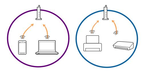
You may not be able to connect to the access point when the access point has multiple SSIDs and devices are connected to different SSIDs on the same access point. Connect the computer or smart device to the same SSID as the printer.
