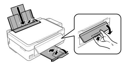
10. Unhook the ink tank unit from the printer and lay it down, and then make sure to install the cap onto the ink tank securely.
