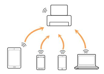
The printer can be connected by Wi-Fi and Wi-Fi Direct (Simple AP) connection simultaneously. However, if you start a network connection in Wi-Fi Direct (Simple AP) connection when the printer is connected by Wi-Fi, the Wi-Fi is temporarily disconnected.
