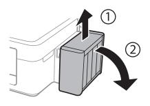
6. Open the ink tank unit cover, and then remove the cap of the ink tank.
