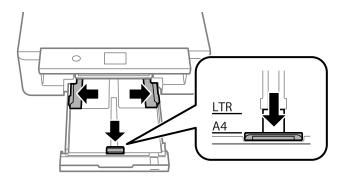
5. With the printable side facing down, load paper until it touches the back of paper cassette.
