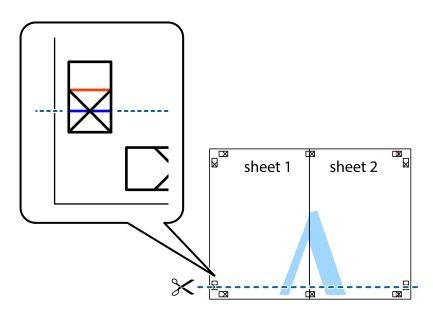
7. Place the edge of Sheet 1 and Sheet 2 on top of Sheet 3 and Sheet 4 and align the cross marks, and then temporarily tape them together from the back.
