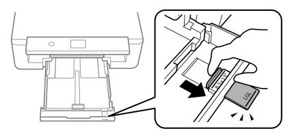
6. With the printable side facing down, load the paper up to the line.
