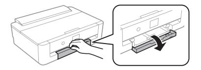
3. Check that the printer is not operating, and then slide out the paper cassette.
