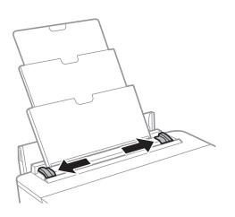
3. Load paper at the center of the rear paper feed with the printable side facing up.
