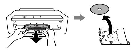
2. Insert the CD/DVD tray back into the slot on the bottom of the paper cassette.
