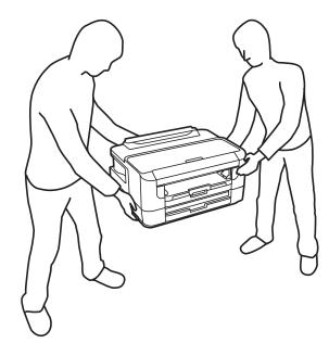
☐ When carrying the printer, do not tilt it more than 10 degrees; otherwise the printer may fall.
