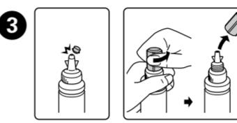
Snap off the top of the cap or remove the cap cover.
