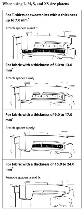
\* The values indicated are when using a grip pad covered platen. When using a platen without grip pad attached, the media you are printing on can be 1.0 mm thicker.
