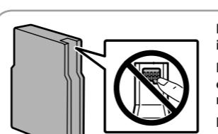
Do not touch the sections shown in the illustration of the cartridge.
