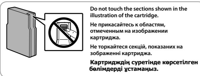
Do not touch the sections shown in the illustration of the cartridge.
