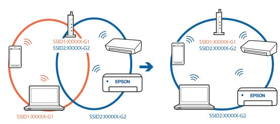
□ A wireless router that is compliant with both IEEE802.11a and IEEE802.11g has SSIDs of 2.4 GHz and 5 GHz. If you connect the computer or smart device to a 5 GHz SSID, you cannot connect to the scanner because the scanner only supports communication over 2.4 GHz. Connect the computer or smart device to the same SSID as the scanner.
