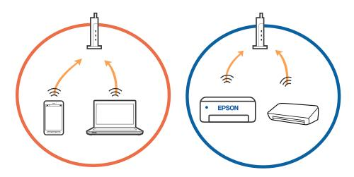
□ You may not be able to connect to the wireless router when the wireless router has multiple SSIDs and devices are connected to different SSIDs on the same wireless router. Connect the computer or smart device to the same SSID as the scanner.
