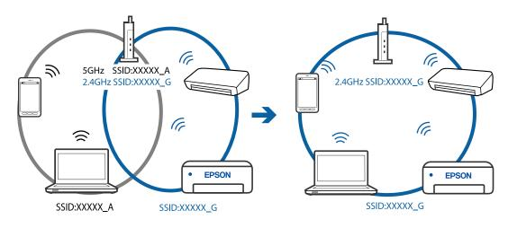
□ Most wireless routers have a privacy separator feature that blocks communication between connected devices. If you cannot communicate between the scanner and the computer or smart device even if they are connected to the same network, disable the privacy separator on the wireless router. See the manual provided with the wireless router for details.
