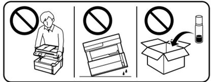
**!** Be sure to keep the ink bottle upright when tightening the cap. Place the printer and the bottle in a plastic bag separately and keep the printer level as you store and transport it. Otherwise ink may leak.
