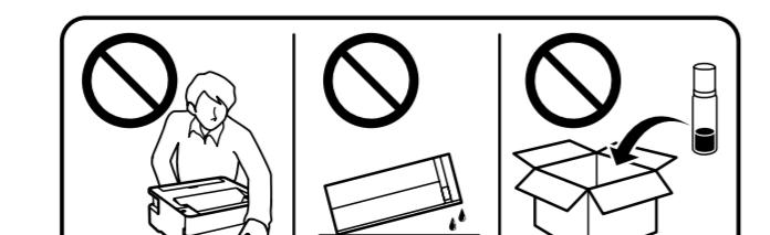
**!** Be sure to keep the ink bottle upright when tightening the cap. Place the printer and the bottle in a plastic bag separately and keep the printer level as you store and transport it. Otherwise ink may leak.
