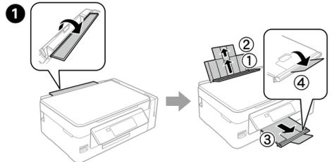
Flip the feeder guard, and then slide out the paper support and the output tray.
