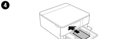
Load paper with the printable side face-down until the paper touches the end of the cassette.
