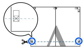
Lay the upper sheet on top of the lower sheet. Lineup the X marks as shown in the illustration below, and temporarily fasten them using an adhesive tape on the back.
