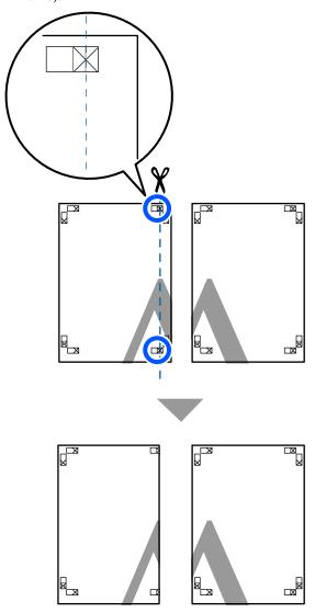
Lay the upper left sheet on top of upper right sheet. Lineup the X marks as shown in the illustration below, and temporarily fasten them using an adhesive tape on the back.
