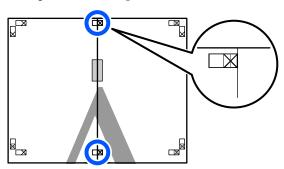
With the two sheets overlapping, trim the excess by cutting along the line joining the two cut guides (the lines to the left of the X marks).
