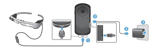
When the battery is charged 90% or higher, the LED indicator stops flashing and remains on. The LED indicator turns off when the battery is fully charged. (The LED indicator provides a rough indication of the amount of remaining battery.)
