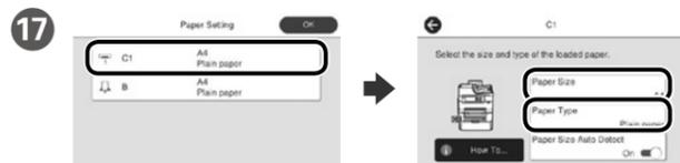
Check the paper size and paper type for the paper sources. Tap **OK** if the settings are correct, or select the correct paper size and paper type. You can change these settings later.
