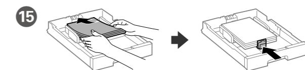
Load A4 size paper toward the back of the paper cassette with the printable side face down then slide the front edge guide to the paper.
