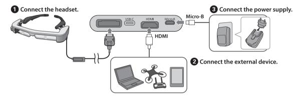
When using the headset sensor or camera data, connect to the USB-C port. Video signals from the HDMI port have priority over video signals from the USB-C port.
