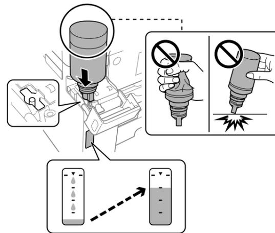
If the ink does not start flowing into the tank, remove the ink bottle and try reinserting it.
