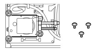
9. Connect the two cables to the circuit board.
