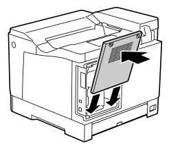
12. Secure the rear cover with the two screws.
