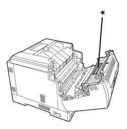
You can see the duplexing unit and the duplexing unit cover by opening the front cover using button B. The asterisk (\*) indicates the position of the caution label.
