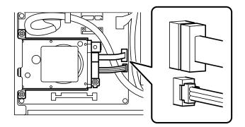
10. Secure the cable with the clamp.
