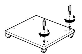
3. Set the lowest paper cassette unit on the printer stand. Align each of the holes on the bottom with the guide pins.
