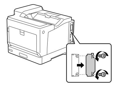
Install the ethernet board straight into the additional interface slot for the ethernet board. Insert the ethernet board firmly into the slot.
