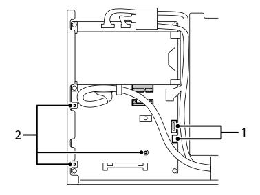
5. See the following to identify where to place the HDD.
