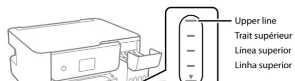
**4** Insert the ink bottle straight into the port to fill ink to the upper line.
