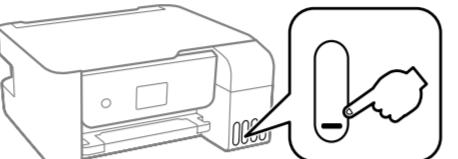
To confirm the actual ink remaining, visually check the ink levels in all of the printer's tanks. Prolonged use of the printer when the ink level is below the lower line could damage the printer.
