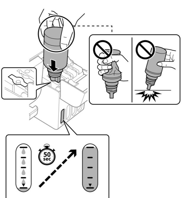
**When you insert the ink bottle into the filling port for the correct color, ink starts pouring and the flow stops automatically when the ink reaches the upper line.**
