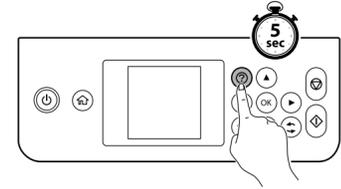
**12** Confirm that the tanks are filled with ink, and then press the **⏻** button to start charging ink. Charging ink takes about 11 minutes.
