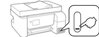
To confirm the actual ink remaining, visually check the ink levels in all of the printer's tanks. Prolonged use of the printer when the ink level is below the lower line could damage the printer.
