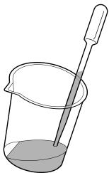
Drip some cap cleaning liquid (2 to 3 drops) from the dropper until the inside of the anti-drying caps (all the caps except the left edge) are full.
