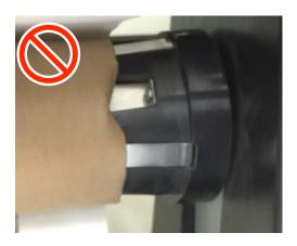
☐ Depending on the paper type and paper width, the paper may become misaligned with the roll or too loose and then cause Reel Unit Error when taking up over a long distance.
