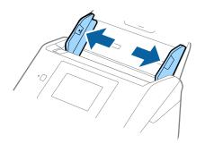
Load the laminated cards into the input tray facing down with the top edge facing into the ADF.
