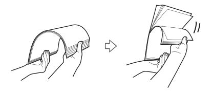
4. Align the edges of the originals with the printed side facing down and slide the leading edge into a wedge shape.
