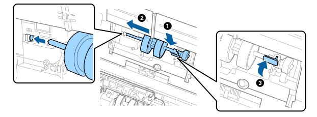
7. Put the edge of the cover of the pickup roller into the groove and slide it. Close the cover firmly.
