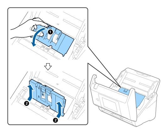
4. Open the cover of the pickup roller, and then slide and remove it.
