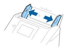
3. Place the Carrier Sheet with the illustration on the front edge facing up and place the photo in the center of the Carrier Sheet with the side to be scanned facing down.
