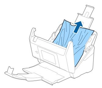
4. If you cannot pull originals straight up, carefully pull out any jammed originals from the output tray in the direction of the arrow.
