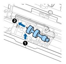
10. Insert the new separation roller axis into the hole on the right side, and then lower the roller.
