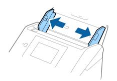
3. Load the originals at the center of the input tray in descending order of paper size with the widest at the back and the narrowest at the front.
