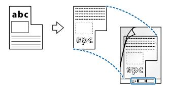
Load the Carrier Sheet into the input tray with the top edge facing into the ADF.
