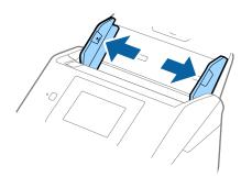
3. Place the Carrier Sheet with the illustration on the front edge facing up and place the original in the center of the Carrier Sheet with the side to be scanned facing down.
