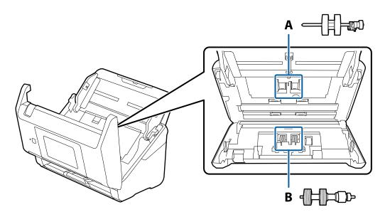
A: pickup roller, B: separation roller
