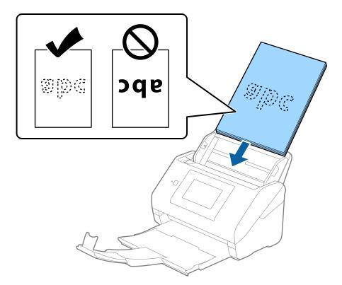
6. Slide the edge guides to fit the edge of the originals making sure there are no gaps between the originals and the edge guides. Otherwise, the originals may be fed skewed.
