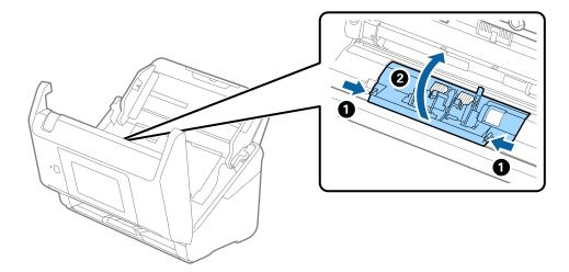
9. Lift the left side of the separation roller, and then slide and remove the installed separation rollers.
