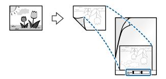
Load the Carrier Sheet into the input tray with the top edge facing into the ADF.
