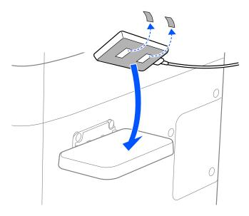
5. If the clamp has not been installed in the printer, peel off the seal from the printer, and then insert the clamp.
