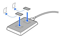
4. Peel off the seals on the double-sided tape, and then secure the authentication device to the authentication device table.
