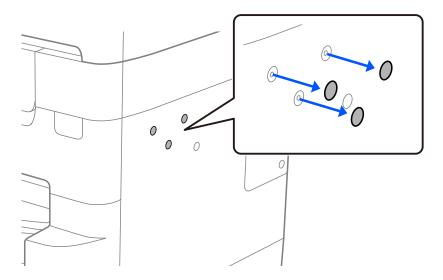
2. Use a coin or a screwdriver to secure the base plate with the screws.
