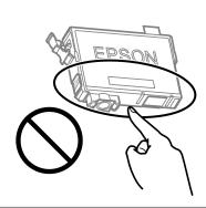
$^{5\cdot}$  Squeeze the tab on the ink cartridge and pull it straight up. If you cannot remove the ink cartridge, pull it firmly.
