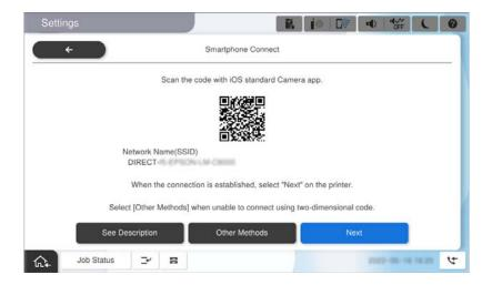
5. On your iPhone, iPad or iPod touch, start the standard Camera app, and then scan the QR code displayed on the printer's control panel in PHOTO mode.
