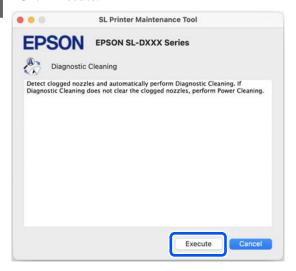
The nozzle check starts and cleaning is executed if necessary.
