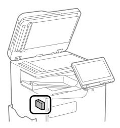
3. Use the cleaning cloth to clean the surface of the scanner glass.
