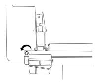
3. Slide and remove the cutter blade unit from the cutter unit, then attach the new cutter blade unit.
