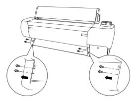
3. Hold the cutter unit, and hook its left side to the left square hole on the platen.
