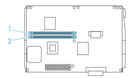
5. Hold the memory module above the memory slot and insert it into the slot until the clips come up to hold the memory module securely in place. Do not apply too much force.
