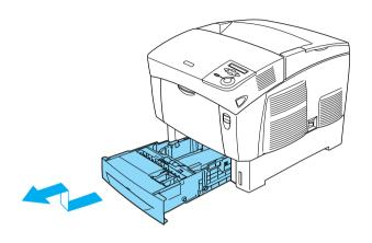
2. Slide the guides to accommodate the paper you are loading. Tilt the rear guide forward to slide it.
