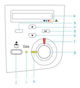
a. LCD panel Displays printer status messages and control panel menu settings.
