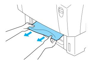
*Note:* Confirm that the jammed paper is not still deep inside the printer.
