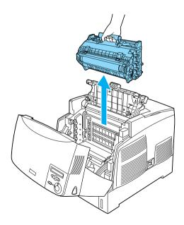
5. Take the new photoconductor unit and tear away the top portion of the bag along the dotted line to expose the handle. Then, grab the handle and remove the styrofoam insert and tear open the bag along the dotted line.
