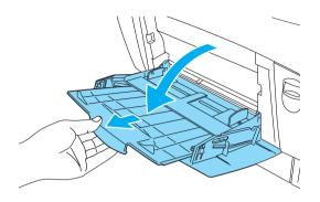
2. Load a stack of the desired media with the printable surface facing down, then slide the guides against the sides of the stack to get a snug fit.
