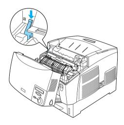
4. Unlock the locks on both sides of the fuser unit.
