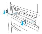
9. Remove the cover on the back of the standard lower cassette, and secure the back of the unit to the printer with the remaining two screws. Then reattach the cover.
