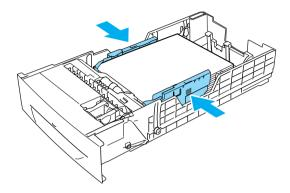
6. Insert the paper cassette gently into the printer, and push it back it the printer.
