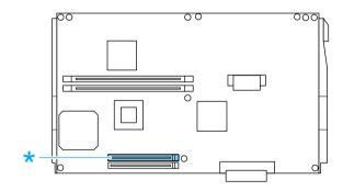
6. Push down on the tab on the right side of the ROM slot to raise the module out of the slot A.
