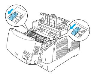
5. Lift the fuser unit out of the printer as shown below.
