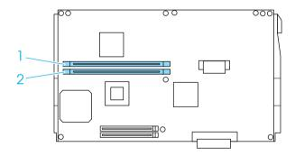
6. Grasp both sides of the memory module and pull the module out.
