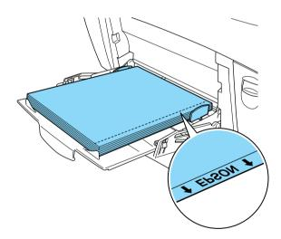
If transparencies are loaded incorrectly, the message Check Transparencies appears on the LCD panel. Remove the transparencies from the MP tray and remove the jammed transparencies from the MP tray. Open and close cover A to clear the message on the LCD panel, then reload the transparencies. The printer resumes printing from the page that jammed.
