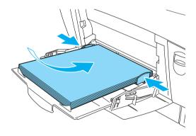
3. Select the Paper Source and Paper Size settings that match the loaded media by using the printer driver or the printer's control panel.
