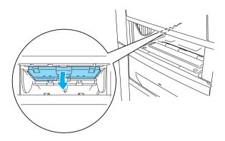
When the paper jam is cleared completely and cover A is closed, printing resumes from the page that jammed.
