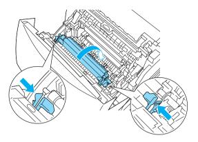
3. Pull the transfer unit out of the printer.
