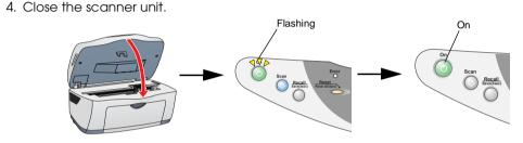
Ink charging starts. It takes about two minutes. While charging, this product produces a variety of mechanical sounds. This is normal. When the **On** light stops flashing, ink charging is complete
