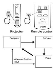
**3.** Press the Source button on the projector or the Computer, S-Video or Video button on the remote control to select the video source you wish to project.
