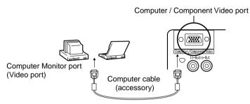
\* If your computer port style is not a mini D-Sub 15-pin interface, use a connection adapter that provides this interface.
