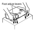
**1.** Support the projector unit with your hands, pull upward on the foot adjust levers with your fingers, and lower the unit slowly.
