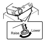
**4.** Make fine adjustments to the height. Turn the lower portion of the front adjustable feet to make fine adjustments to height.
