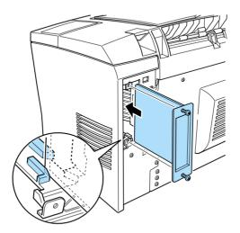
4. Secure the interface card with the two retaining screws.
