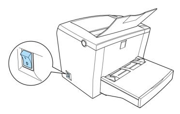
2. Insert the power cord into the back of the printer and plug the other end into a properly grounded electrical outlet.
