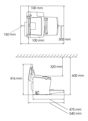
□ If you install the optional 500-Sheet Lower Paper Cassette Unit, you will need an additional 125 mm (4.9 inches) in height. If you install the optional Face-up Tray, you will need an additional 150 mm (5.9 inches) at the back of the printer.
