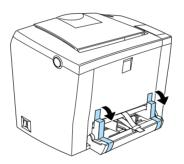
6. Pull the protective plastic strip straight out of the MP tray slot as shown above. It is necessary to pull firmly to remove this protective material.
