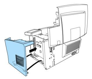
7. Fasten the side cover with the two screws.
