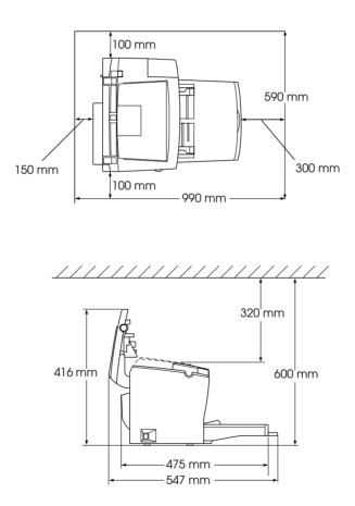
□ If you install the optional 500-Sheet Lower Paper Cassette Unit, you will need an additional 125 mm (4.9 inches) in height. If you install the optional Face-up Tray, you will need an additional 150 mm (5.9 inches) at the back of the printer.
