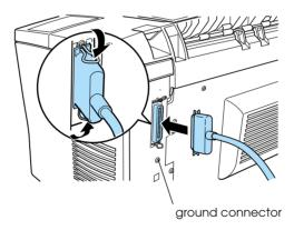
3. Plug the other end of the cable into the computer's parallel interface connector. If there is a ground wire at the computer end of the cable, connect it to the ground connector at the back of the computer.
