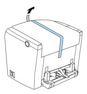
5. Remove the two protective tape strips and the L-shaped plastic foam pieces from the front of the printer.
