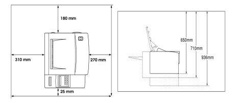
☐ If you install the optional Duplex Unit (see "Installing the Optional Duplex Unit" on page 4), you will need to allow an additional 235 mm (9.3 inches) at the back of the printer.
