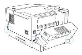
6. Use the supplied clips to fasten the duplex unit to the printer and close the duplex unit's vertical unit. Make sure the clips are fastened securely.
