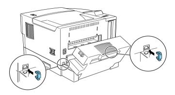
7. Completely remove the paper cassette. Pull out the duplex unit feeder tray until you can see the two feeder joints at the front of the printer.
