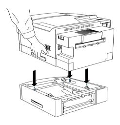
4. Lower the printer and duplex unit combination onto the 500 sheet lower paper cassette, taking care to line up the corners. Make sure that the printer and duplex unit are firmly seated.
