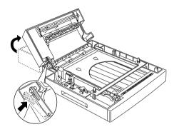
2. Remove the transparent cover attached to the rear of the printer. Insert the duplex chute into the body exit of the printer, and secure it with the two supplied clips.
