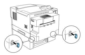
6. Completely remove the duplex feeder tray and pull out the 500 sheet lower paper cassette until you can clearly see the two feeder joint areas on the duplex unit.
