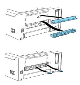
3. Inside the vertical unit, you will find a metal bar. Use this bar to remove the plastic cover at the right of the body exit.
