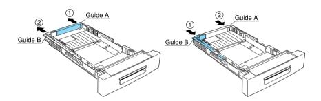
5. Fan a stack of paper (up to 250 sheets) to separate the sheets, and tap the edges of the stack on a flat surface to even up the edges. Insert this stack of paper into the cassette, lining it up with the left side of the cassette. Make sure that all sheets of the stack are under the metal retaining clip and the plastic tabs on the end guides. If you overload the cassette by putting too many sheets of paper in at one time, this can cause paper jams.
