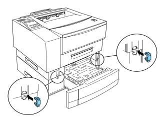
8. Push the 500 sheet lower paper cassette back in and replace the duplex feeder tray.
