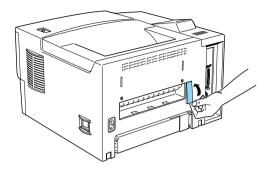
When you have removed the plastic cover, store it together with the metal bar in the place in the vertical unit where you found the metal bar.
