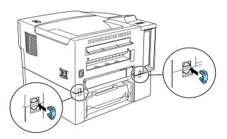
6. Remove the upper 250 sheet paper cassette completely from the printer, and pull out the lower 500 sheet paper cassette until you can see the front feeder joints.
