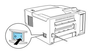
3. The printer warm up and several messages appear on the display as the printer performs tests. After about 45 seconds, and after a short while, the display will show Ready.
