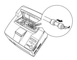
4. With a clean damp cloth, wipe the pickup roller's rubber parts.
