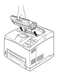
3. Take the new imaging cartridge out of its package and gently shake the imaging cartridge as shown below.
