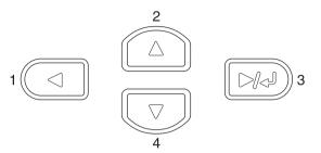
11. Press the Down button to display Reset Fuser Counter, and then press the Enter button.
