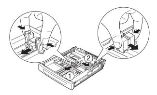
4. Load a stack of the desired media on the center of the cassette with the printable surface facing up. Then slide the side paper guide while pinching the knob until it is against the right side of the stack to get a snug fit.
