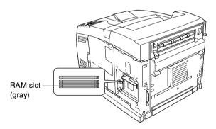
5. Insert the memory module into slot until the clip lock onto the memory module. Make sure that the left slot (white) has a module at all times.
