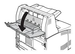
2. Remove any paper you find jammed inside the Stacker as shown in the illustration below.
