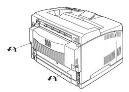
3. Press the unlock button to unlock the hooks, then remove the unit from the printer.
