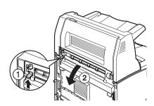
4. Remover the screws on both sides of the Stacker, and while holding up the Stacker, remove the right and left tabs from the holes on the top of the printer.
