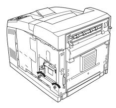
6. Connect one end of the cable that comes with the Hard Disk Drive to the socket on the Hard Disk Drive.
