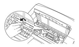
4. Gently pull out any sheets that have fed part way into the printer.
