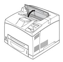
2. Hold the handle of the imaging cartridge and pull out.
