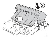
6. Secure the screws at both ends of the bottom of the stacker.
