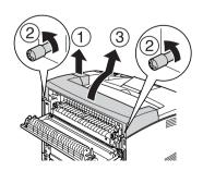
5. Insert the right and left tabs of the Stacker into the holes on the top of the printer and slowly lower it onto the top of the printer.
