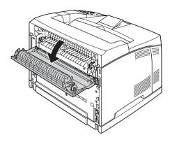
4. Pull down the two levers at either side of the fuser unit.
