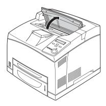
2. Hold the handle of the cartridge and pull it out.
