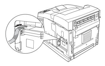
8. Insert the bottom side of the Hard Disk Drive into the printer and push it to set it in the correct position.
