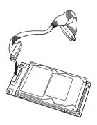
7. Connect the other end of the cable to the Hard Disk Drive socket on the circuit board.
