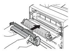
7. Lift up the two levers at either side of the fuser unit and push down the levers at both ends of the fuser unit to lock it.
