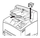
3. Lift up the second lever at the top left corner of the back of the printer to open cover B.
