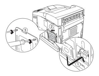
7. Reattach the right side cover to the printer as shown below. Then, tighten the screw on the back of the printer.
