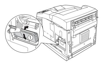
9. Secure the drive with the screws. Use the screw that comes with the drive to secure the upper-right corner, then use the two screws that you removed in step 5 to secure the positions you took them out of.
