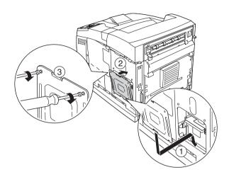
11. Reattach the right side cover to the printer as shown below. Then, tighten the screw on the back of the printer.
