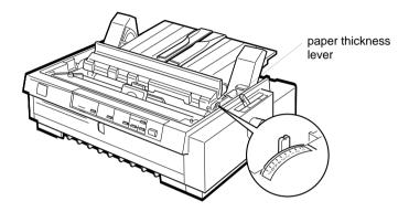
Use the following table to set the paper thickness lever to match the thickness of your paper.
