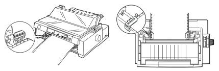
In the standby position, your paper is attached to the printer but is not inside the printer.
