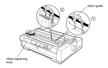
10. Turn the ribbon-tightening knob in the direction of the arrow to remove any slack in the ribbon as shown in step 9. Then slide the print head from side to side to make sure it moves smoothly.
