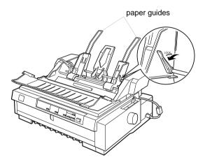
4. Holding the lower portion of the left paper guide, slide it until it is aligned with the arrow mark on the back of the center support. Then push the left lock lever backward to lock it in place. Holding the lower portion of the right paper guide, slide it to match the width of your paper, but do not lock it.
