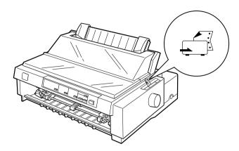
4. Release the left and right sprockets by pushing the sprocket lock levers backward.
