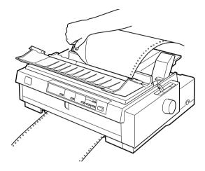
□ Use the **paper release lever** to change the paper path without removing continuous paper from the tractors.
