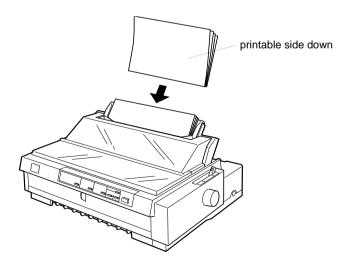
Insert the of form in the front slot, bound edge first and printable side up, as shown below.
