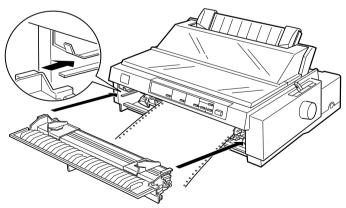
10. Slide the edge guides to the middle of the top paper guide base. Lift the center section of the paper guide base up and lay it flat. Make sure that the printer cover and the paper guide cover are closed.
