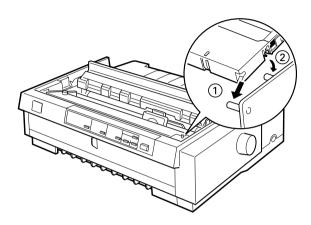
8. Make sure that the two rear notches of the cartridge fit over the small pegs on each side of the printer. Then gently press down the cartridge until both ends click into place.
