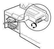
3. If your cable has a ground wire, connect it to the printer's ground connector as shown below.
