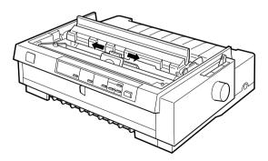
11. Replace the printer cover by first inserting the front tabs into the slots on the printer and then lowering the cover into place. Push it down until it clicks.
