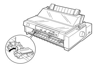
5. Slide the left sprocket to the left margin of your paper using the arrow mark inside the printer. (Printing starts at the arrow mark.) Then pull the lever forward to lock it in place.
