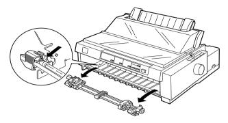
5. Replace the front paper guide by sliding it along the printer's mounting slots until it locks in place. Then close the front paper guide.
