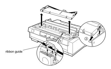
6. Remove the new ribbon cartridge from the package. Then remove the separator from the middle of the ribbon cartridge and discard the separator. Turn the ribbon-tightening knob in the direction of the arrow to remove any slack in the ribbon.
