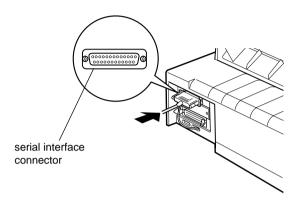
Tighten the screws on the both sides of the connector.
