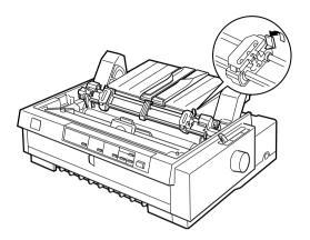
5. Slide the left sprocket to the left margin of the paper using the scale on the paper guide as a guide. (Printing starts at the arrow mark.) Then push the lever back to lock it in place.
