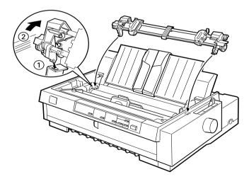
You are now ready to load continuous paper onto the pull tractor as described in the next section. To remove the pull tractor, see "Removing the pull tractor" on page 2-31.
