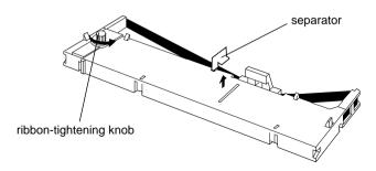
7. Hold the cartridge with the ribbon-tightening knob up. Fit the two front notches of the ribbon cartridge over the small pegs on each side of the printer as shown below. Then lay the cartridge flat.
