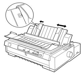
3. Set the paper release lever to the single-sheet position. Also set the paper thickness lever (located under the printer cover) to the proper position for your paper's thickness. (See the table on page 3-3.)
