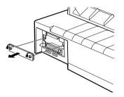
3. Slide the interface card along the slots on both sides of the interface compartment. Firmly push in the card to make sure the connector at the back of the interface card is fully inserted into the printer's internal socket. Then replace the screws and tighten them.
