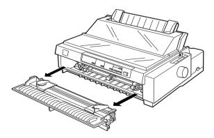
3. Set the paper release lever to the front push tractor position. Also set the paper thickness lever (located under the printer cover) to the proper position for your paper's thickness.
