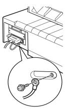
4. Plug the other end of the cable into the computer.
