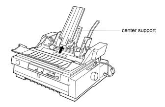
3. Release the left and right paper guides of the cut-sheet feeder by pulling the lock levers forward.
