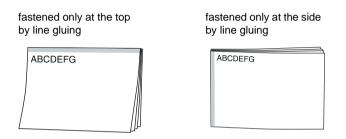
□ You can use the top or front paper slot to load single-sheet multi-part forms that are fastened at the top.
