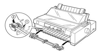
You are now ready to load continuous paper onto the front push tractor as described in the next section. To remove the tractor, see "Removing the front push tractor" on page 2-18.
