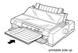
□ You can load single-sheet multi-part forms bound at the side only in the front slot. Insert the of form in the front slot, top edge first and printable side up, as shown below.
