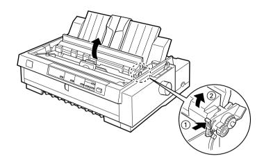
3. Lower the tractor into the printer's mounting slots and press down both ends of the tractor to make sure that it is firmly seated.
