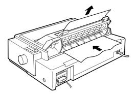
When you finish printing, open the paper guide cover and press the LF/FF button to advance the paper. Tear off the paper using the tear-off edge of the printer (pull it towards you for a clean cut).
